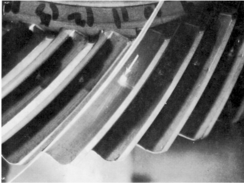
204-040-701 AND 412-040-701 SPIRAL BEVEL GEAR UNACCEPTABLE PATTERN
