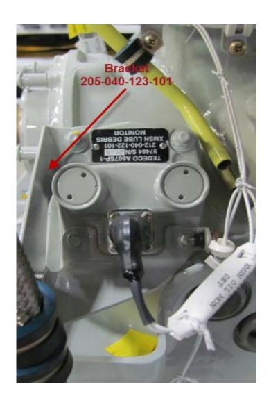
Figure 1 - Full Flow Debris Monitor Correct Installation
