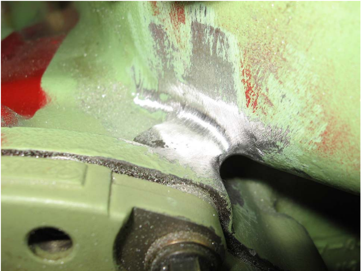
Top side after sanding with Dremel rotary tool
