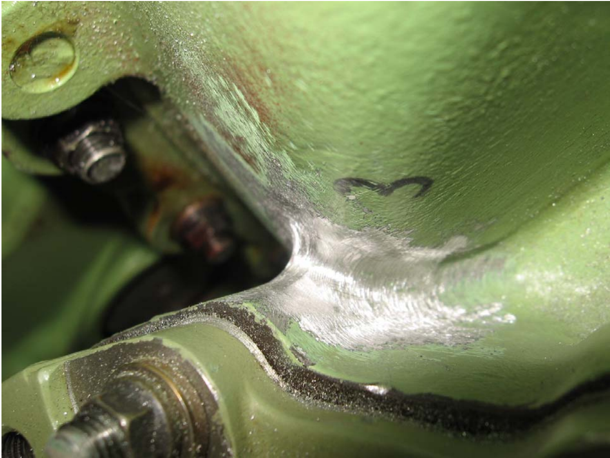
Bottom side after sanding with Dremel rotary tool
