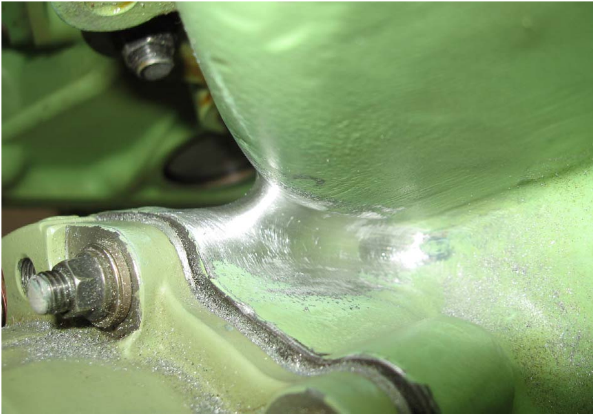
Bottom side after Hand Sanding/Polishing
