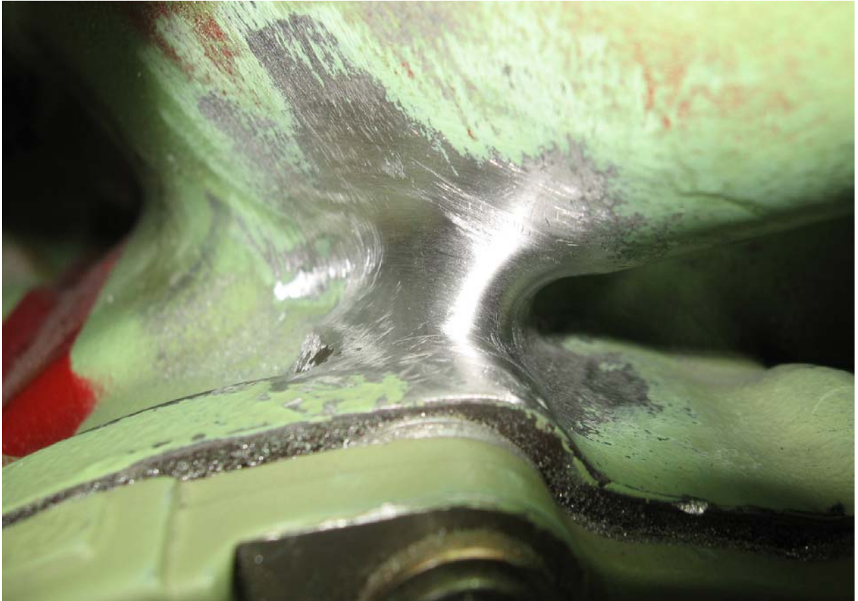
Top side after Hand Sanding/Polishing
