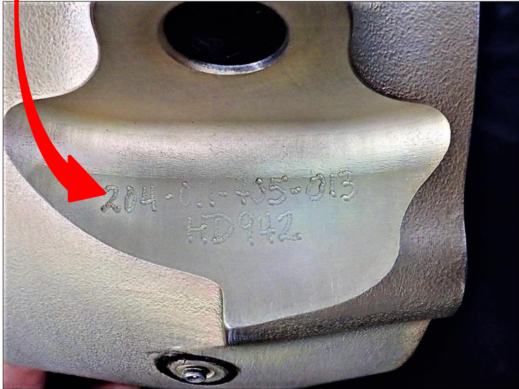
Figure 2 – Vibro-Etched Part Number and Serial Number Location
