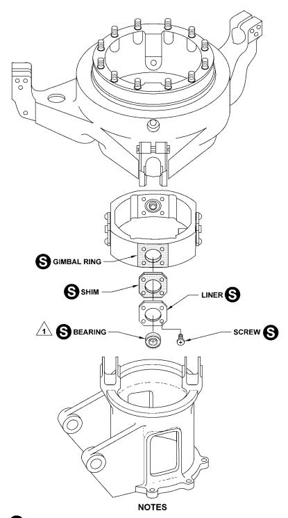
Apply sealant MIL-R-46082, TYPE I (C-352) to faying surfaces as indicated by shading.
