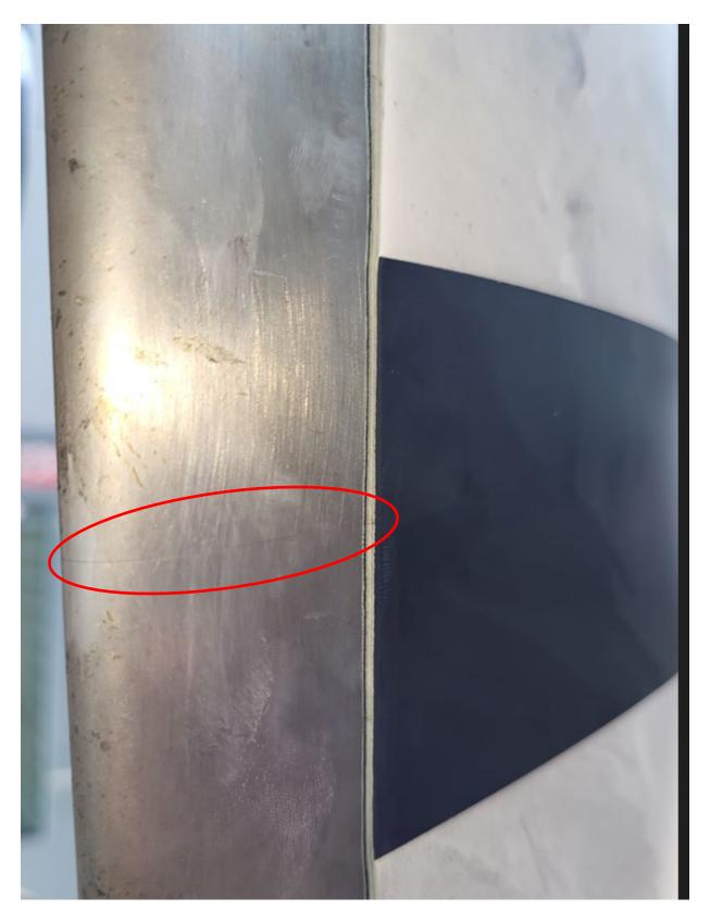
Figure 2 - Example of a Typical Abrasion Strip Crack
