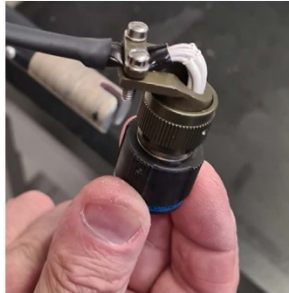
Figure 23 – Locking of the quick clamp connector
