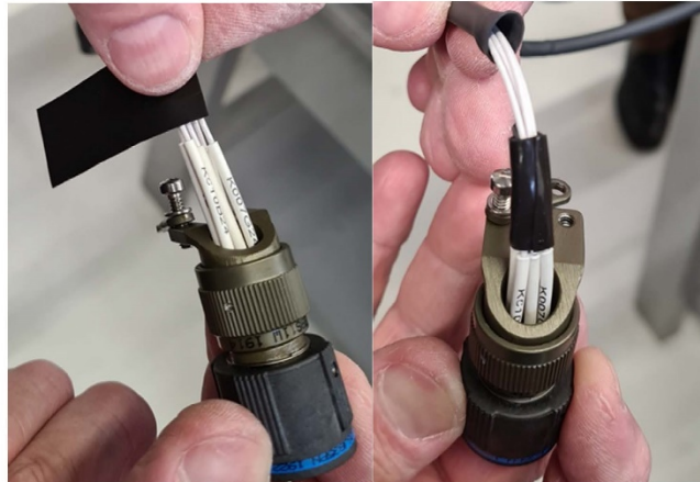
Figure 22 – Installation of the self-agglomerating silicone tape
