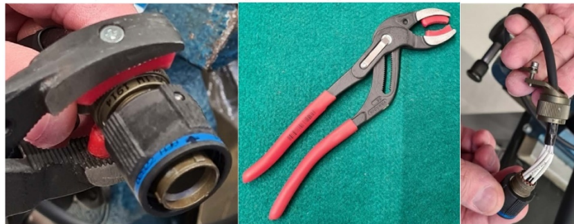
Figure 7 – Removal of the quick clamp connector
