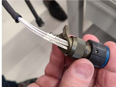
Figure 21 – Installation of the quick clamp connector
