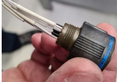
Figure 20 – Installation of the electrical plug connector
