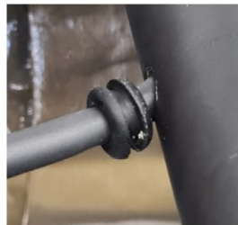
Figure 12 – Removal of the grommet
