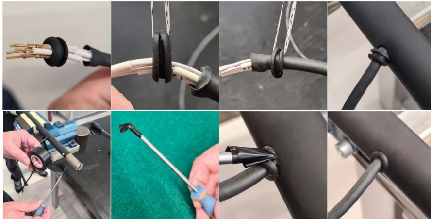
Figure 18 – Installation of the grommet
