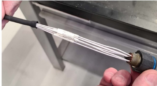
Figure 9 – Getting access to the connector pins
