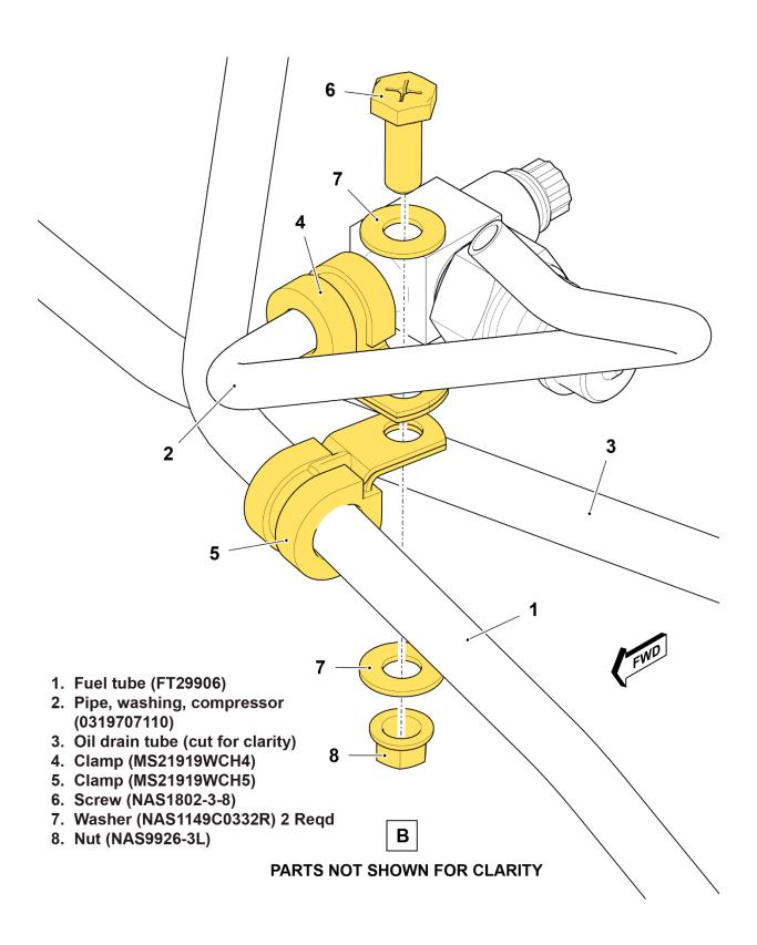
Figure 1 – Installation of clamps (sheet 2 of 2)
