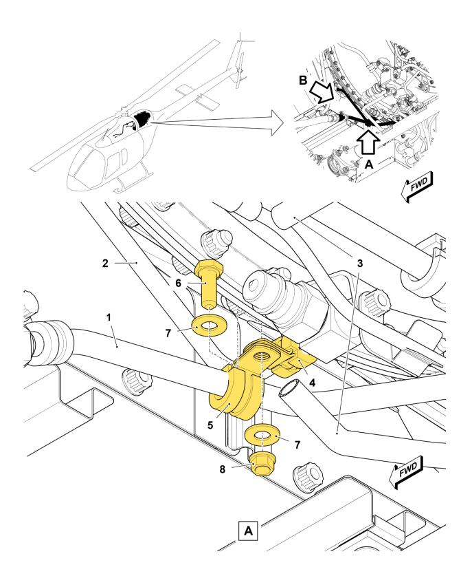
Figure 1 – Installation of clamps (sheet 1 of 2)
