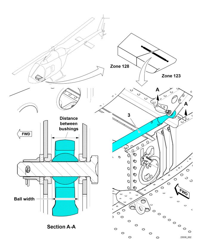
Figure 1 – Cyclic Control Tube and Fixed Support Assemblies (sheet 2 of 4)
