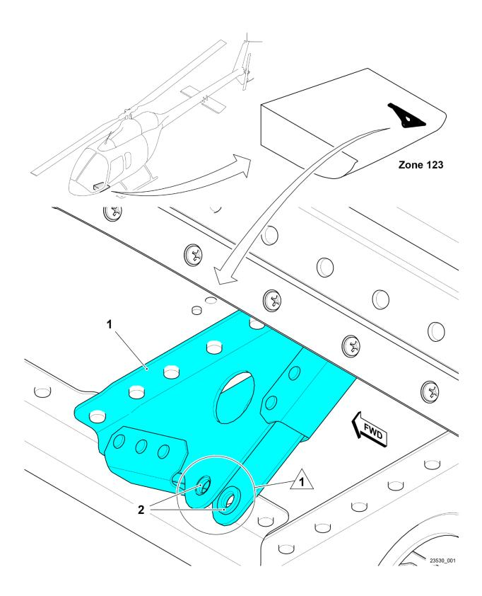
Figure 1 – Cyclic Control Tube and Fixed Support Assemblies (sheet 1 of 4)
