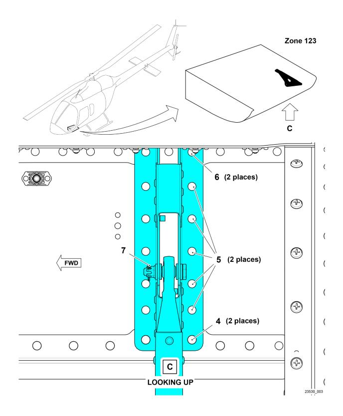
Figure 1 – Cyclic Control Tube and Fixed Support Assemblies (sheet 3 of 4)
