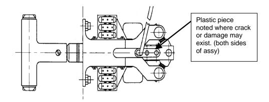
Present inspection intervals require actuation of the Fire "T" Handle to verify serviceability. Bell Helicopter recommends that operators insure that a visual inspection is also accomplished during the required serviceability check to insure cracks are not present. If cracks are detected, the Fire "T" Handle should be removed from service and replaced with a serviceable unit. Report all cracked Fire "T" Handle to Bell Helicopter Product Support.
