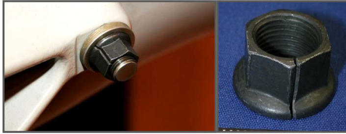
Figure 1: Typical NAS1291 nut application and crack due to hydrogen embrittlement.
