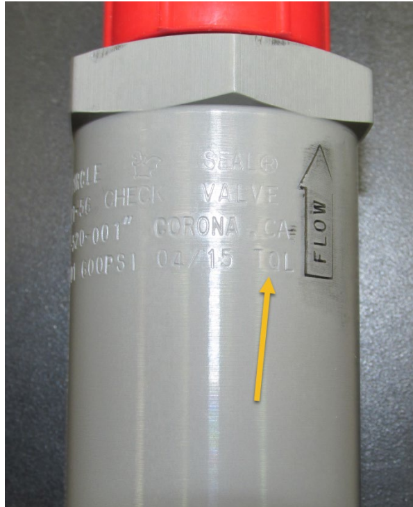
Detail A. Circor Aerospace Engine Oil Check Valve Marked "TQL"
