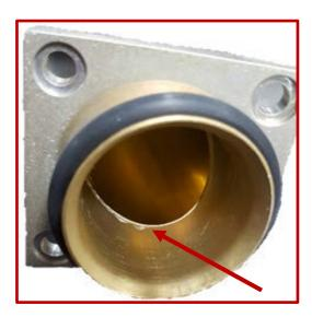
Figure 1 – Examples of Non-Conforming Internal Welds Joints
