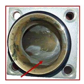
Figure 2 – Example of Internal Weld Joint After Deburring
