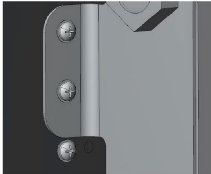
FIGURE 4 – Minimum cut required for screw installation
