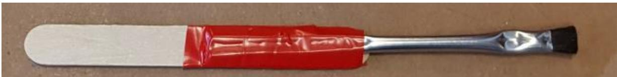
Acid brush used to apply sealant on rivet heads. Bristles can be cut shorter as required.
