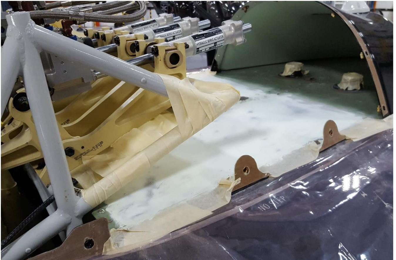
**Figure 5-** Upper roof panels after finishing glaze compound (C-266) application.
