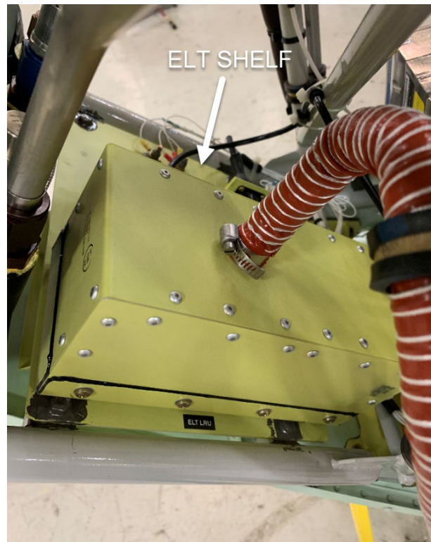
Figure 5 – Emergency Locator Transmitter (ELT) Shelf Brackets (4 places)
